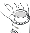
9 Put back the filter basket on the top of the main body.
