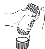
15 The first 8 strokes the pressure is built. Pump slowly until all coffee come out.
