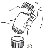
14 Hold the Nanopresso with two hands, as showed above. Start pumping above a cup.
