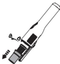
With the dustbin uninstalled, turn counter-clockwise to remove the mesh filter.
