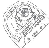
② Remove the inlet filter
