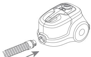
② To remove the hose, hold the main pipe, turn it counterclockwise until it cannot be turned, and then pull out.
