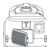
④ Tap the inlet and outlet filters and clean them with water
