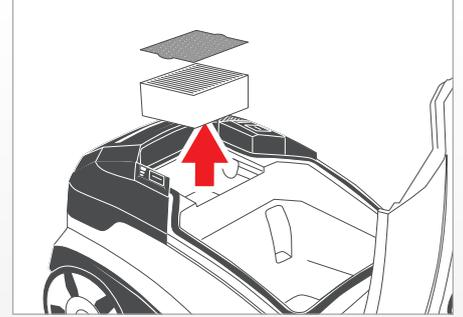
**i** Do not use any brushes or implements which could damage the filter ribs. Allow the two filters to dry before putting them back into the appliance.
