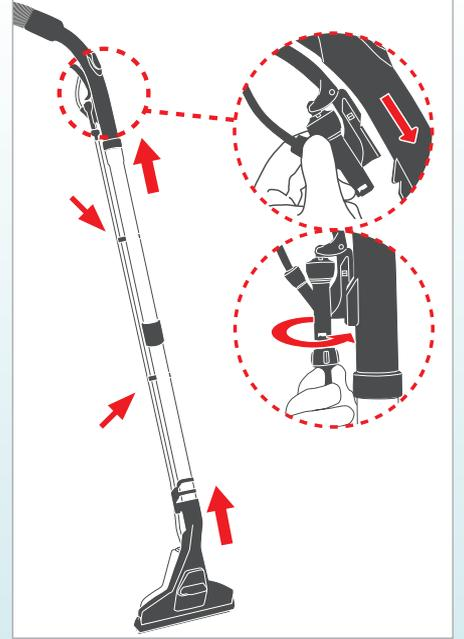
If using the upholstery spray nozzle\*, connect this directly to the handle of the suction hose.
